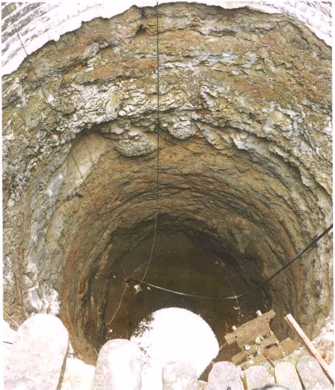
Fractured Basalt Flow below which weathered Compact Basalt Flow is exposed
