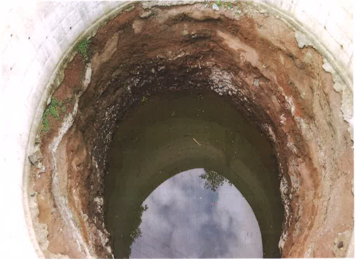
Weathered Basalt below which fractured Basalt flow in exposed
