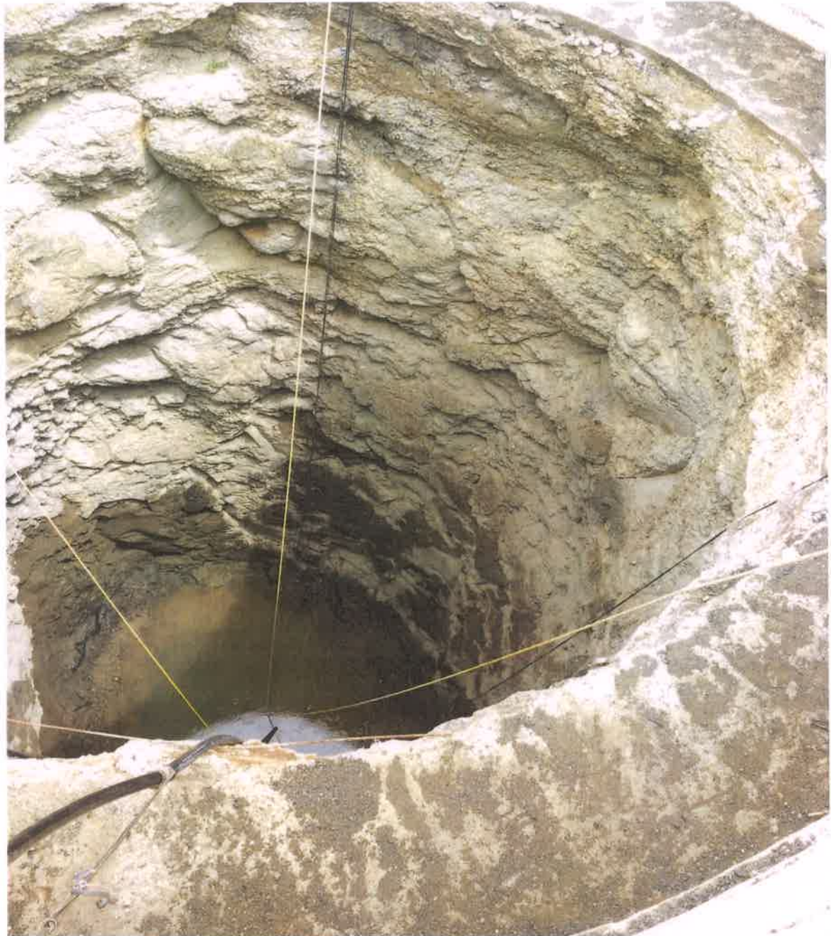
Weathered Compact Basalt Flow with some fractures
