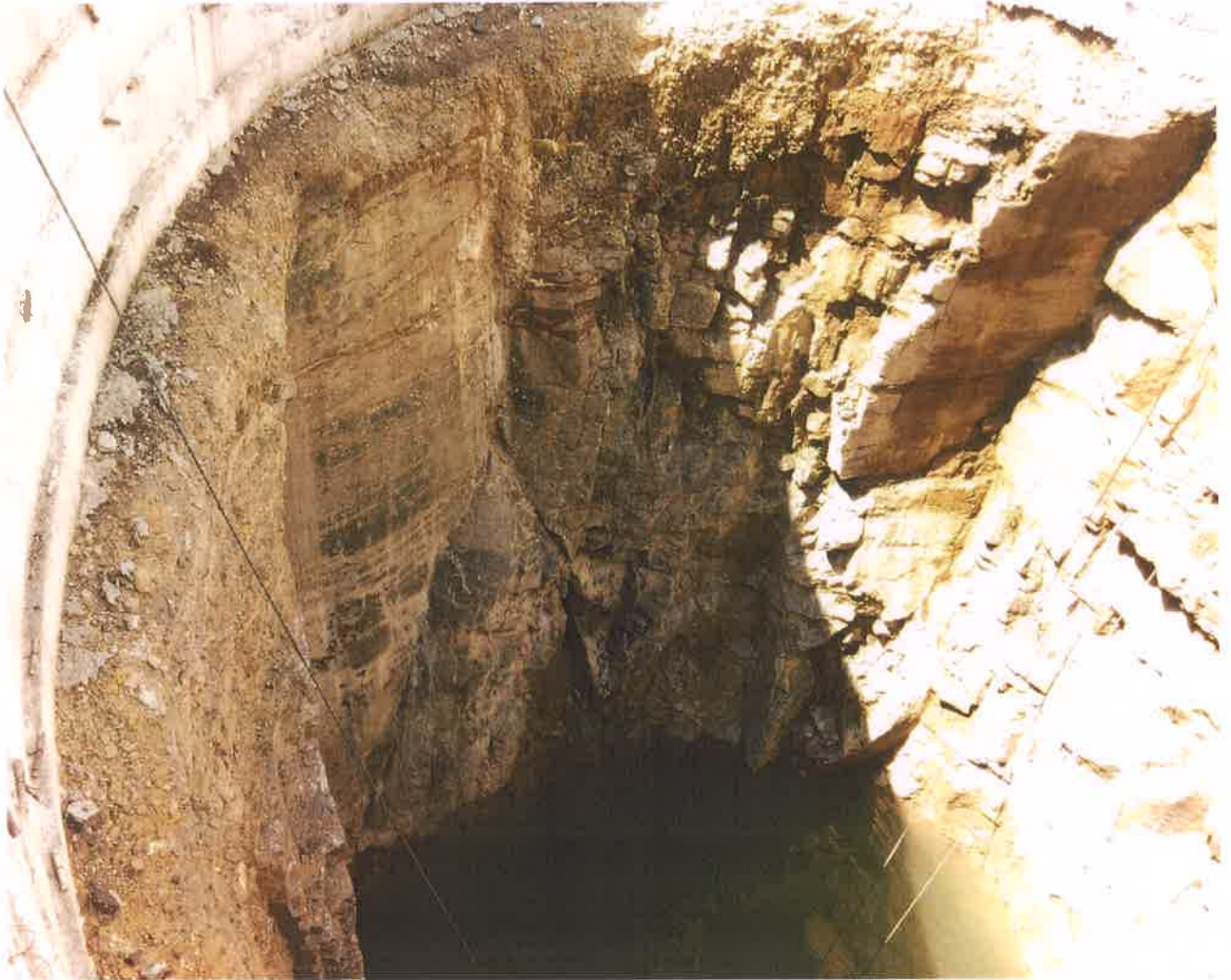
Broadly spaced jointing in basalt flow exposed in the outcrop
