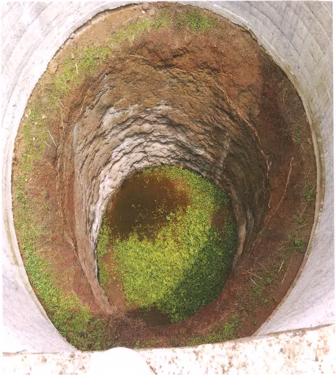
Weathered Compact Basalt can be seen in dug well
